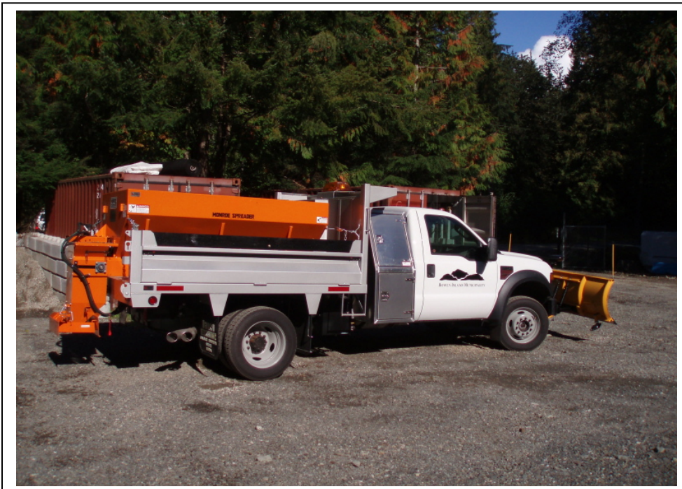
One of our 4WD, 1 Ton trucks fitted with salter/plough combination
