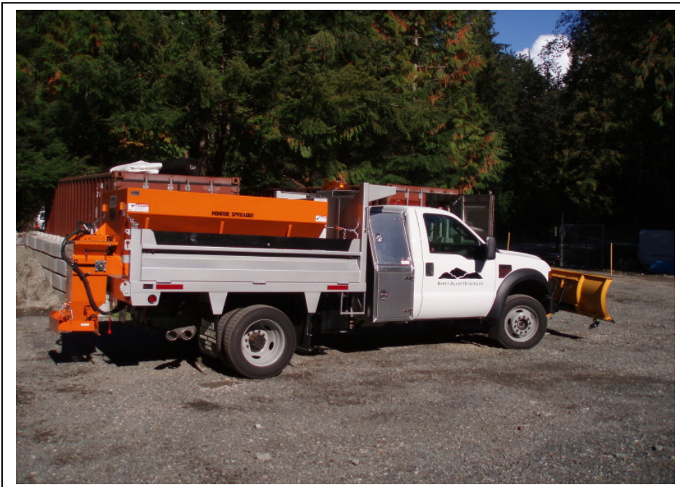
One of our new 4WD, 1 Ton trucks fitted with salter/plow combination
