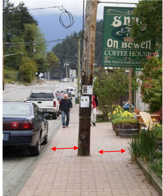
Obstacles in sidewalks, inadequate room for a scooter or wheelchair
